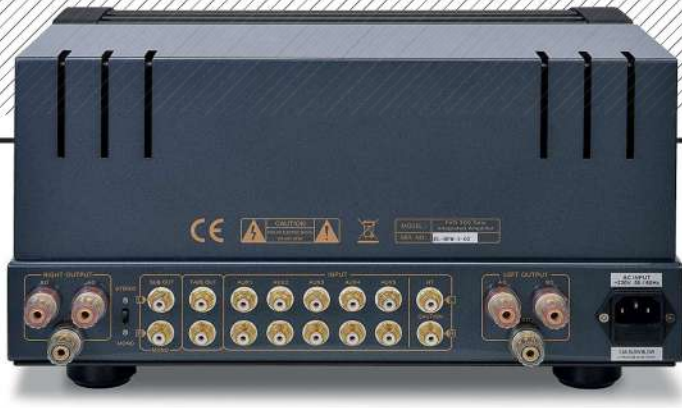
ABOVE: The EVO 300 offers five line inputs, an HT bypass, tape out and sub/mono line outs with a trio of 4mm speaker outputs per channel fed from 8ohm and 4ohm transformer taps, respectively. Optional MM phono module is not shown here
